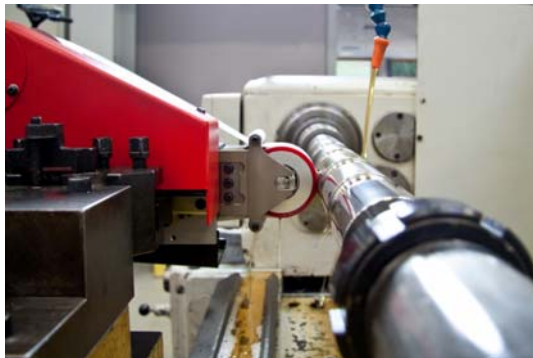
Fig. 4 + 5 Supfina 210 superfinishing attachment on a lathe
